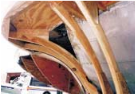
The Londonaire is now Cosmic Muffin . The hull was rebuilt using WEST SYSTEM epoxy.
