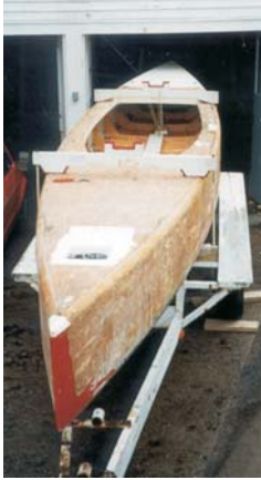
1—My International 110 (Number 300) with the glass and paint removed.
