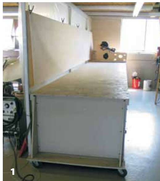
1—This table is used to assemble airplane wings. It must not twist or sag. The table was originally 32' long, but has been shortened to 20'. Four rubber casters, one at each corner, support it. Built as a strongback, it spans 20' (previously 32') without sagging.
