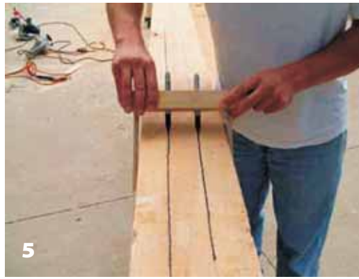
Figure 4—A 2"×8"×24' cap was clamped with metal banding tightened by driving wedges under the bands.
