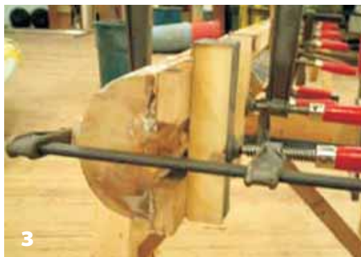
Figure 3—A 1"×2½" piece of Sitka spruce was glued to each side of the cleaned-up fore topmast half to reproduce a hollow area in the center.
