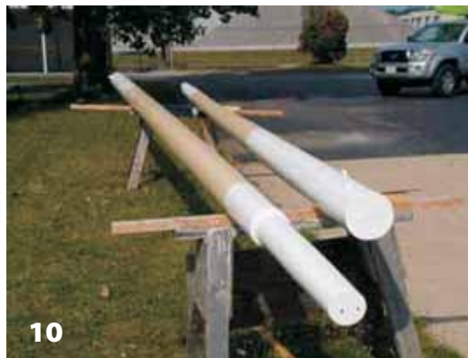
Figure 9—Bill Bauer finish sands a mast. A sanding belt was placed on a drill with a rubber drum to get the final rounding.
