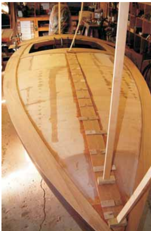
After a slight bit of fairing, the 1/4" mahogany planking was installed. By using the right-sized braces, the roof provided some strategic clamping pressure.
