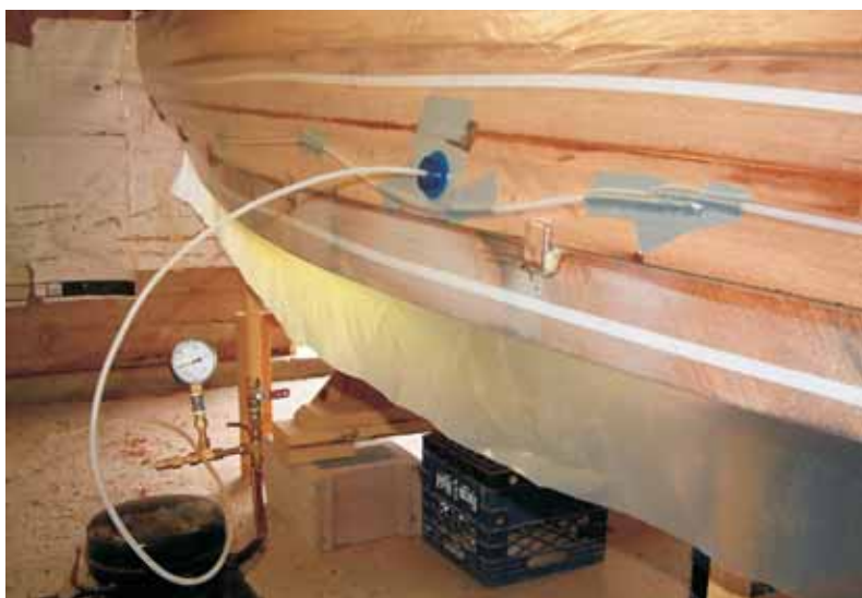
Below right—A closeup of the vacuum port and the clip used to hold the individual planks in position until the vacuum took over.
