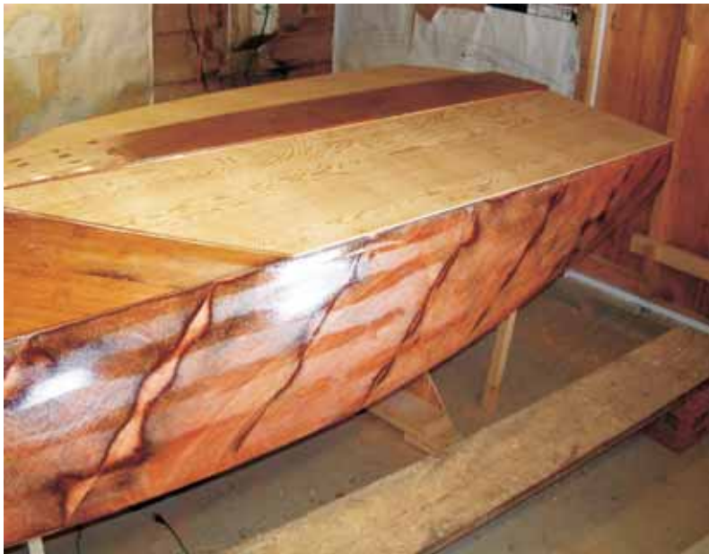
The bottom and topsides are faired and coated, ready for mahogany planking.
