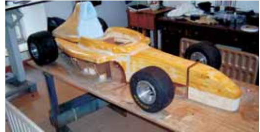
Top —The completed chassis prior to receiving its fiberglass body.
