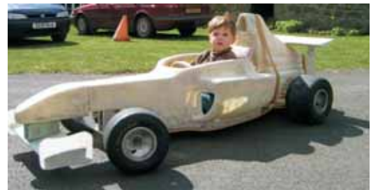
Middle —The plug was designed to come apart in sections. Epoxy/fiberglass body parts were laid up directly on the plug sections, then assembled and faired.
