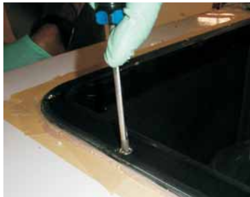
← Photo 5 —Position the hatch over the opening and press it into place, squeezing out any excess epoxy. → Photo 6 —Install the screws, taking care to snug the screws only slightly.
