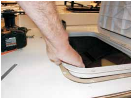
Photo 1—The hatch was easily removed with no damage to the hatch or deck.
