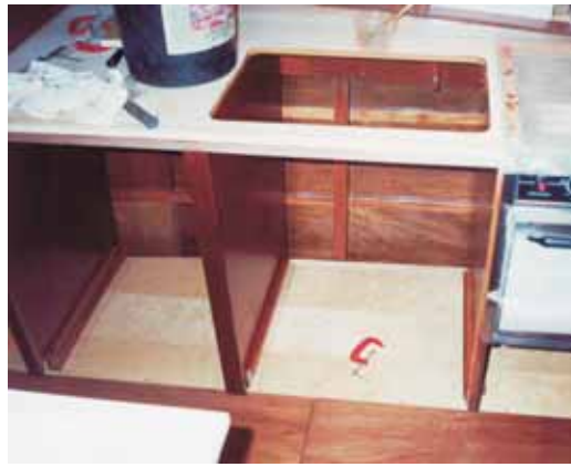
The galley under construction. Throughout 2004 work continued on the interior cabinetry and building of the fuel, water and waste tanks.
