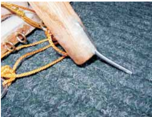
The release pin at the end of the throwing arm allows one end of the sling to release at exactly the right moment, so the tennis ball makes a smooth exit. The pin is a bent nail, glued in with G/5 and wrapped with fiberglass strands saturated with G/5.
