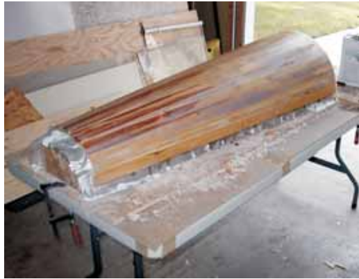
Left—Tapered \frac{3}{8} " thick strips are tacked to the mold. The gaps were then filled with epoxy thickened with 410 Microlight.
