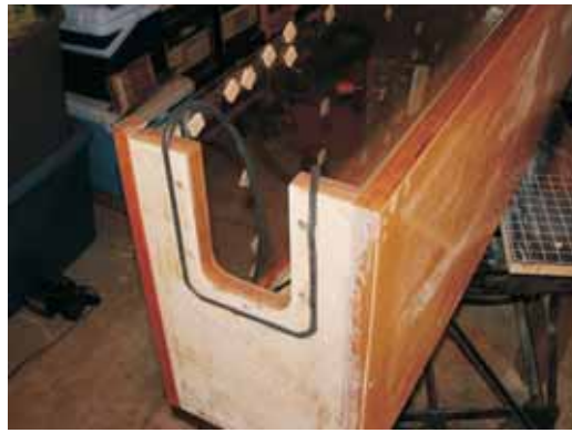
The bolt holes were all located inside of the O-ring seal path to reduce the risk of leakage. Holes were drilled oversized and given a generous coating of epoxy to seal exposed end grain.
