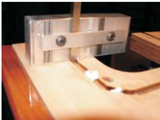
A scraper designed to clean out excess epoxy from the groove that holds the "O" ring. The "O" ring seals the joint between the separate tanks.
