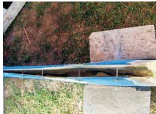
The trailing edge of the rudder was opened up by a hit from a 30-ton whale.
