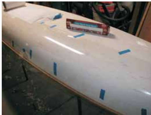
Left —Plastic food wrap stretched over the bottom of the hull to create a non-stick mold surface from which four fiberglass deck parts were made.
