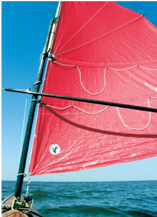
The unique “batwing” gunter rig on Hugh Hor- ton’s Bufflehead .
