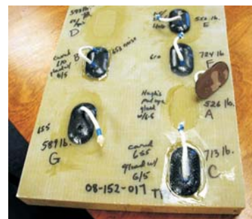
The extraction devise with a digital load cell (left) that recorded the pull off strength of soft pad eyes glued to a fiberglass laminate (right).
