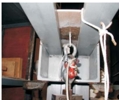
The extraction devise with a digital load cell (left) that recorded the pull off strength of soft pad eyes glued to a fiberglass laminate (right).
