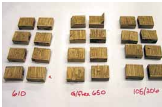
White oak short-block shear test samples after testing to failure. All samples resulted in 100% wood failure.
