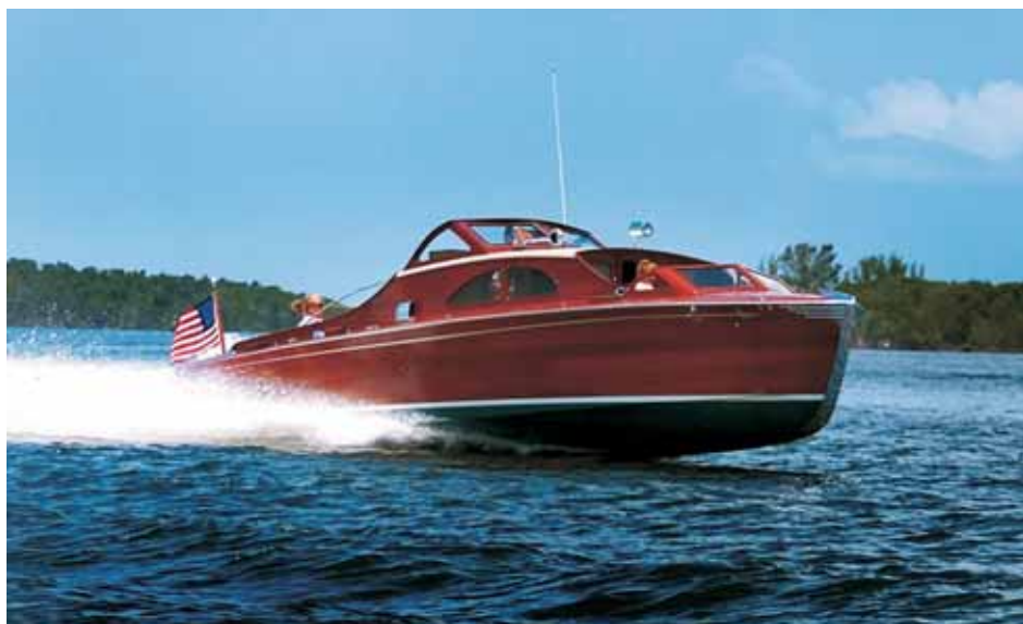
The Charlie Janace designed 36' Commuter has a 9' beam and a 2' 10" draft. It will reach 50 mph thanks to twin 496hp Crusader HO engines.
