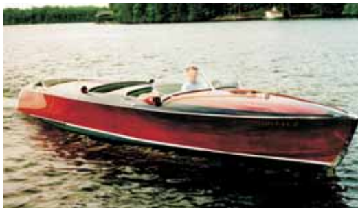
The 27' Sheerliner shown here is powered by a 510 hp V-12 BPM marine engine to achieve a 60 mph top speed.
