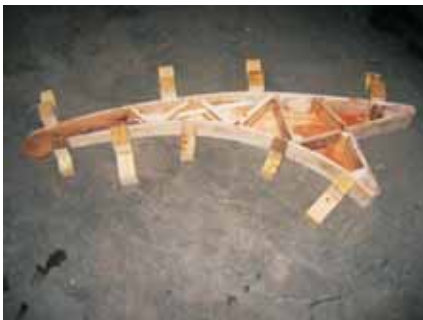
Clamping block served as a "stuffing jig" Compression struts connected top and bottom laminate to create a truss.
