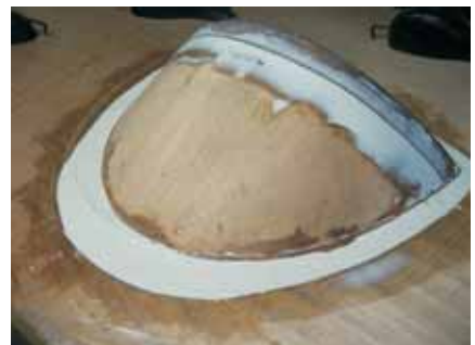
The sink was bonded into the counter cutout.
