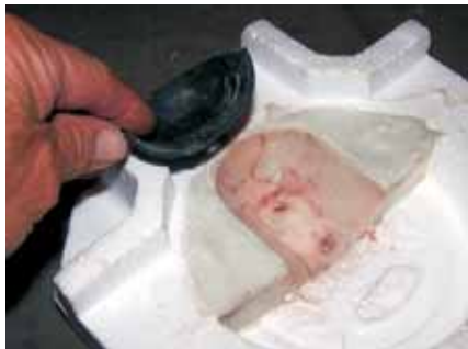
The cap left a good impression of itself in the cured epoxy.
