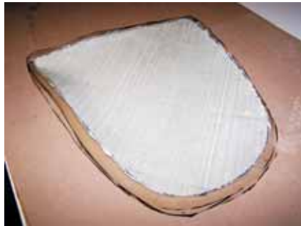
738 Biaxial fabric with mat ready to be wet out with epoxy, placed between sheets of plastic and molded to shape when the epoxy gels.
