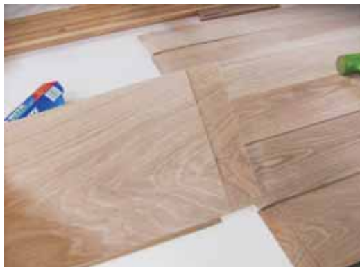
Left—Stepped scarf to help align the stock while making full-length plies.
