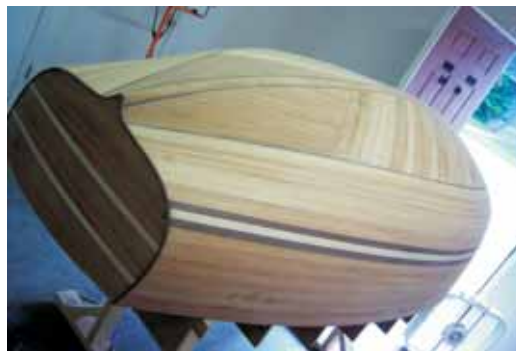
The stripped dinghy hull before glassing still looks pretty good in a raw state.
