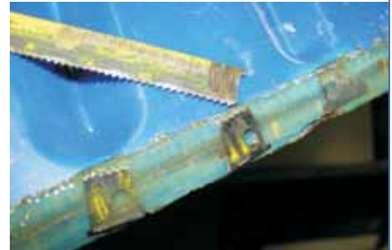
The new and improved wear strips made of hardened steel.
