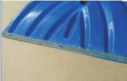
The working edge of my trusty blue shovel with the wear strips worn through.
