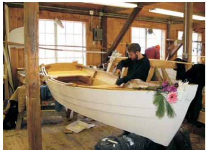
Traditional carvel or lapstrake are the construction methods used most often at The Apprenticeshop. Students here are working on a traditional lapstrake dory.
