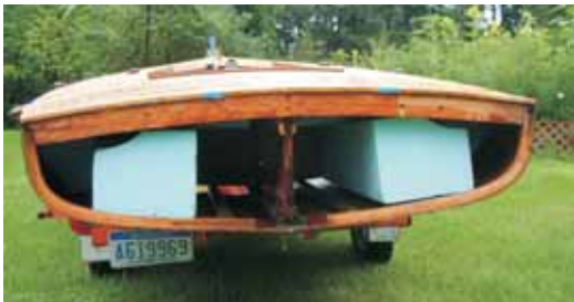
The remaining part of the transom was removed to reveal a nice solid frame.
