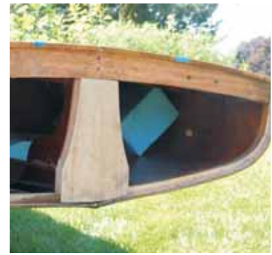
Left—The transom gusset clamped with a handy 4 × 4.
