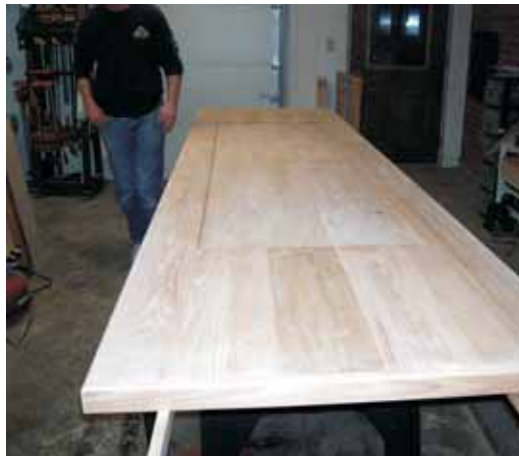
The oak bar top ready for a sealer coat of epoxy. Note the recessed center where the pour will go.
