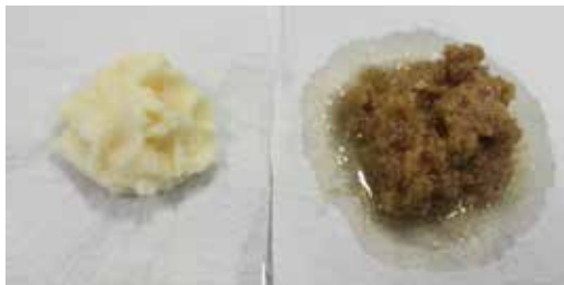
On the left is epoxy mixed with our 406 Filler. On the right is epoxy and sanding dust mixed to the same consistency as the filler. Notice the puddle of epoxy draining out of the epoxy/sanding dust mixture.
