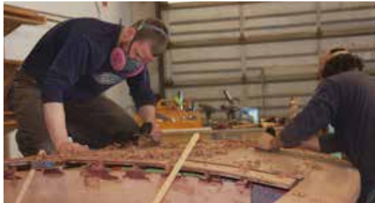
The deck consists of 1/4" plywood bonded with epoxy to the deck frames followed by mahogany deck strips. In this photo you can see both the plywood underlayment and the mahogany decking as it gets planed smooth by Ben Van Dam and Chad Buras.
