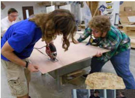
The students worked in teams of 3 to cut out the patterns (above) and assemble them (right) with the stitch and glue technique.
