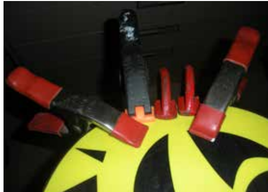
Spring clamps and a couple C clamps were used to exert the right amount of pressures for a strong repair.
