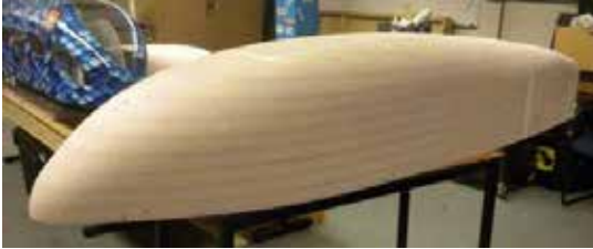
Figure 1.3 - Male mold plug constructed from 2 inch thick foam sheets.
