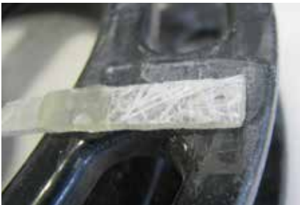
G/flex Epoxy was used to adhere the fiberglass ring to the reel face.
