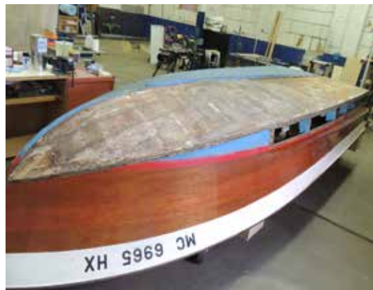
The boat rolled over with half of the bottom removed.
