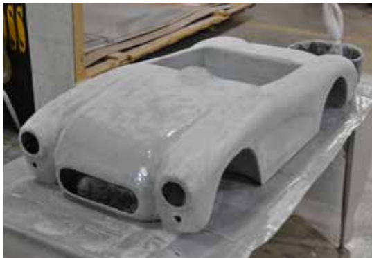
The fiberglass was coated with thickened WEST SYSTEM Epoxy and 503 Gray Pigment.
