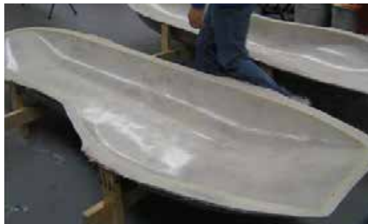
Figure 1.4 - Female mold with left and right halves built with WEST SYSTEM Epoxy and 404 High Density filler
