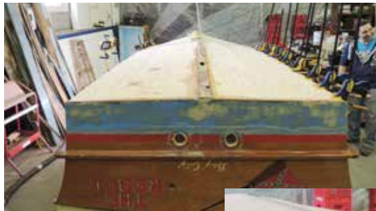
The bottom of the boat restored with new plywood (above) and the reinstalled and new mahogany planking (right).
