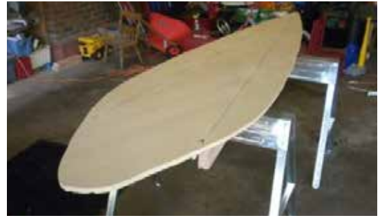
Figure 1.5 - Platform used to keep foam sheets from warping during assembly
