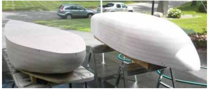
Figure 1.8 - Upper and lower plug sections separated following final sanding.
