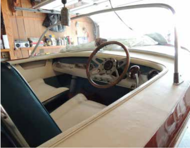
The seat and the new dash reinstalled complete the restoration of the neglected Chris Craft.
