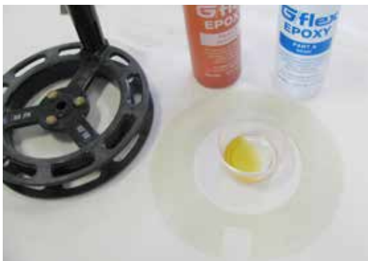
G/flex Epoxy was used to adhere the fiberglass ring to the reel face.
