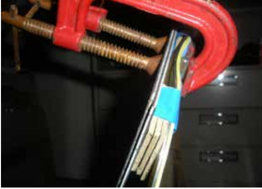
A C clamp, shims, and a metal backer plate were used to straighten the damaged area before gluing back together.
