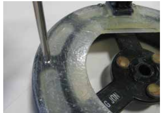
Screws were used in addition to gluing as an added reinforcement.
