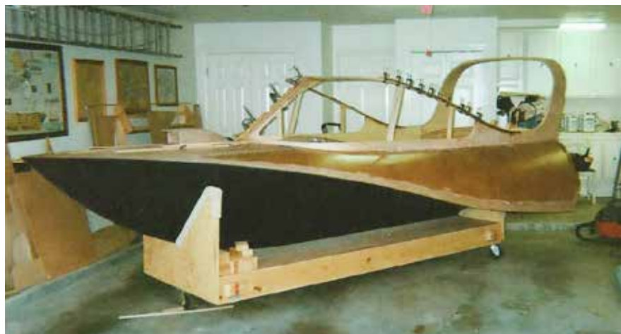
The windshield frame and its bracing in the final stages of laminating.
