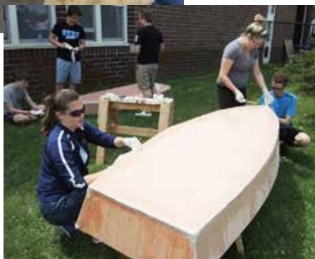
The students worked in teams of 3 to cut out the patterns (above) and assemble them (right) with the stitch and glue technique.
