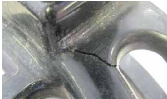
The cracks in the nylon plastic needed to be reinforced before they completely failed.
