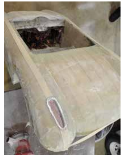
The plug shaped and over-laid with WEST SYSTEM 105/205 epoxy and fiberglass cloth.
