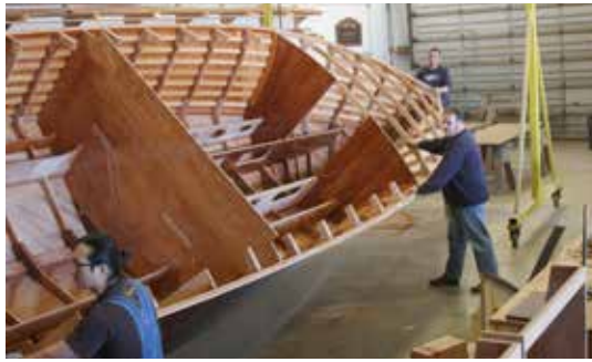
The rolling of the Limousine begins. Large eye hooks fore and aft are used to secure the belts during the roll. Steve Kim and Michel Berryer control the boat as it's rolled.
