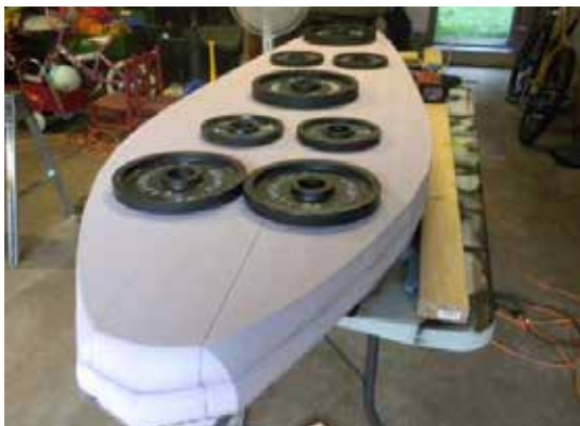
Figure 1.6 - Sheets are stacked and held in place with weights prior to fastening with 3" screws
