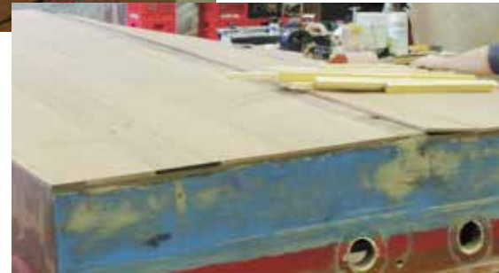
The bottom of the boat restored with new plywood (above) and the reinstalled and new mahogany planking (right).
