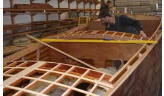
The deck consists of 1/4" plywood bonded with epoxy to the deck frames followed by mahogany deck strips. In this photo you can see both the plywood underlayment and the mahogany decking as it gets planed smooth by Ben Van Dam and Chad Buras.
