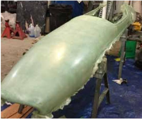
*An exact copy of the borrowed car body was created from the female mold.*
