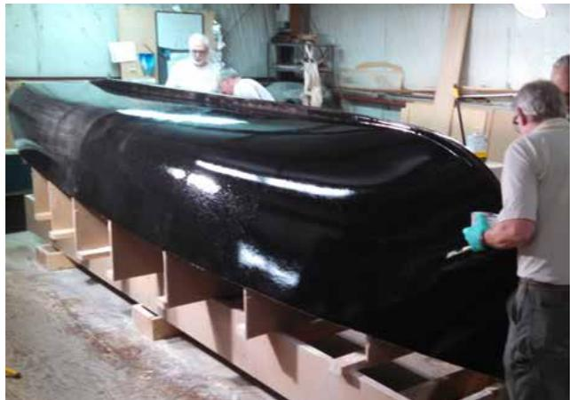
*The hull off the mold and covered with fiberglass. The interior was faired before the fiberglass was applied.*
