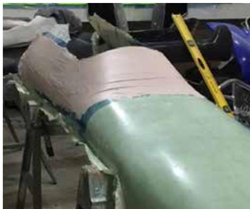
*A fairing compound was applied over the flash tape to smooth the surface and stiffen the area. This will be sanded fair and sealed with epoxy.*
