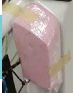
The final mold shape covered with packing tape to make a smooth surface
