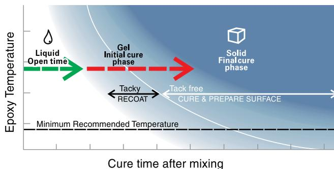
As it cures, mixed epoxy passes from a liquid state, through a gel state, to a solid state.
