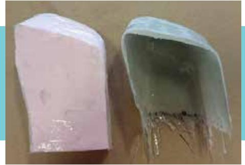
Mold removed from the cured epoxy/fiberglass part
