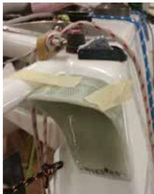
Sanded, trimmed part being fit in place
