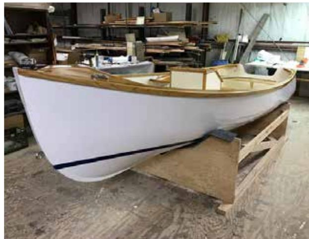
*With the interior painted, the hardware was installed. It's important to seal all holes with epoxy after they are drilled.*
