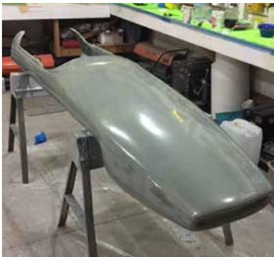
*An old car body was loaned to be used as a plug to create a female mold.*
