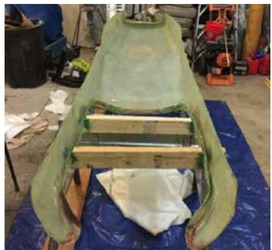
*Because the loaned car body could not be altered, this female mold was created to build a second body that could be altered.*
