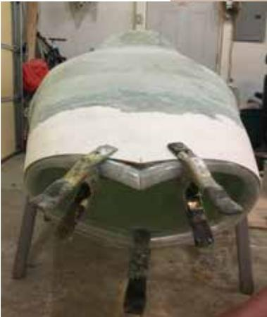
*A scrap of curved fiberglass panel was the perfect piece to extend the nose of the car body to match the new profile.*
