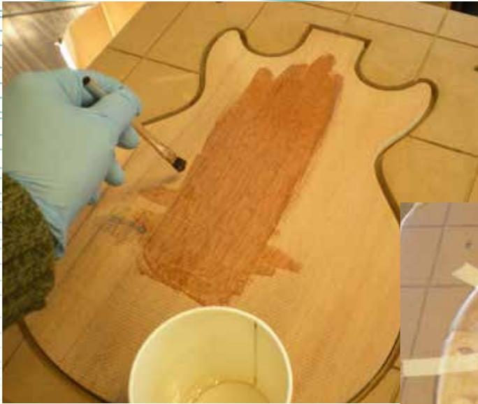
*105/207 is being applied for bonding the marquetry work. Using 105/207 to adhere the marquetry and as the seal coat, gives the finished product a unified appearance.*
