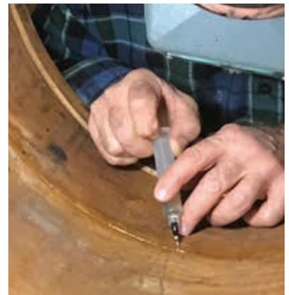
WEST SYSTEM 105/205 was injected directly into the crack and clamped to cure.
