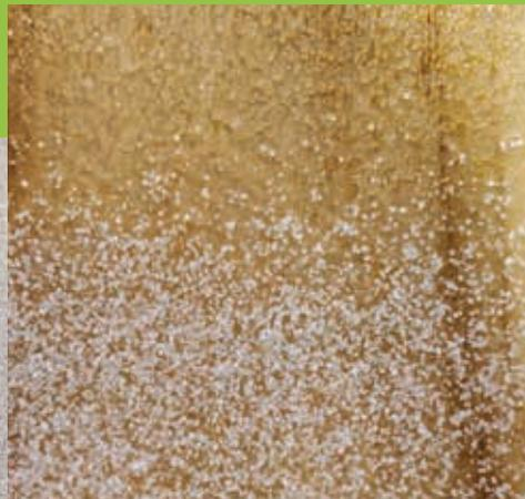
you want. The tests need to be completed all the way to painting the topcoat. Keep in mind that it can be difficult to abrade a textured epoxy surface, but this is necessary so that the paint will adhere to the epoxy and protect it from UV exposure (which degrades all epoxies over time). A 3M Scotch Brite™ pad or a wire bristle brush can be helpful when trying to abrade the epoxy's textured surface.
