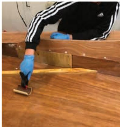
*After brushing the epoxy on, Joshua tipped the coat with a section of a 300 Roller Cover with a clamp for a handle.*
