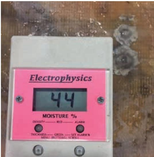
*A moisture meter measures the conductivity within a laminate and therefore can be helpful in determining where there is saturated core.*
