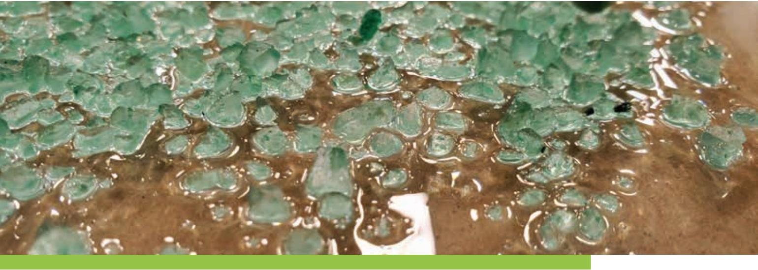
Rock salt used for the lost method of creating nonskid.
