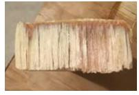
An example of a successful bond. The bonding of the epoxy to the plywood was stronger than the bond of the wood fibers to one another. You can see the wood fibers still attached to the end of the 2x4.
