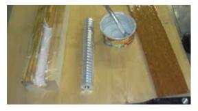
mechanical holding power. He used WEST SYSTEM Epoxy thickened with 404 High-Density filler to attach the aluminum rod, then covered it with a wooden cap. This method ensures the outside of the bar is encapsulated in epoxy and there are no
