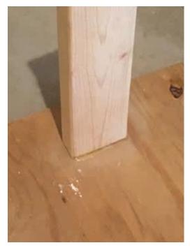
An example of a home adhesion testing setup. The end of a 2x4 was epoxied onto the surface of a plywood panel and allowed to fully cure.
