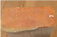
This timber bonded unsuccessfully. You can see the shine of the epoxy on the bottom of the 2x4. Note that there are no wood fibers missing from the plywood panel in the top image or attached to the end grain in the bottom image.
