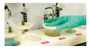
The peak exothermic temperature is measured using 100 cc of epoxy in a standardized 120 cc beaker. A thermocouple connected to a computer analyzes the results.
