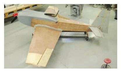
for the spar on this plane. He decided to use hard maple and transition to Douglas fir towards the outer edges of the wing spar. The idea was to keep the strain at failure for the spar similar throughout its cross section.
