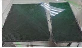
Two of the panels for the switches and gauges. The finished surface was carbon with green metallic accents woven through the fabric.
