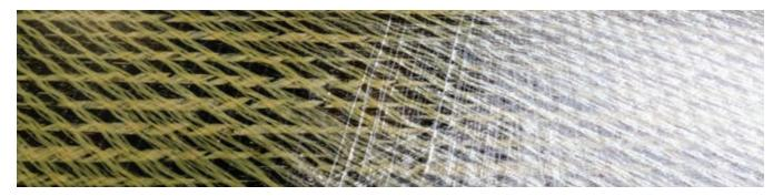
impact and abrasion resistance. Because of their high strength, they're frequently used in sailboat rigging. Honeywell Spectra fabrics tend to be more expensive, so might not be as readily available as other reinforcement fabrics in retail settings.
