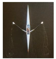
Bob Cole built this Colin Angus Cambridge Racer recreational rowing shell using WEST SYSTEM® Epoxy. The shell is 23' 3" long and weighs 39 lbs. The hull and deck are 3mm Okoume.
