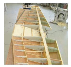
The wing was built with fiberglass/aluminum honeycomb ribs bonded onto a plywood skin.
