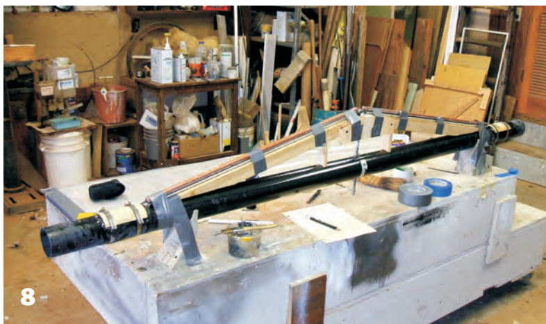
8—Carbon beams were purchased from Ben Hall and then a carbon dolphin striker was added to the front beam.
