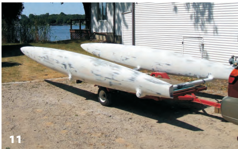
11—The faired catamaran upside-down on a trailer. Gluing the beams to the hulls rather than bolting them on resulted in a very stiff platform.
