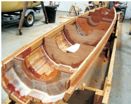
Above—Half of a glued column removed from the building frame.
