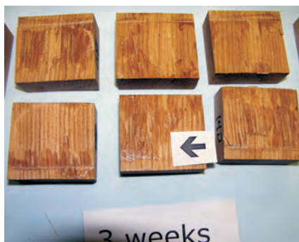
The arrow is pointing to some shiny epoxy found in a three-week 105/205 sample. Close examination showed that it was not a cohesive failure-both matching areas were shiny, which indicates a void. This sample was not included in the average.
