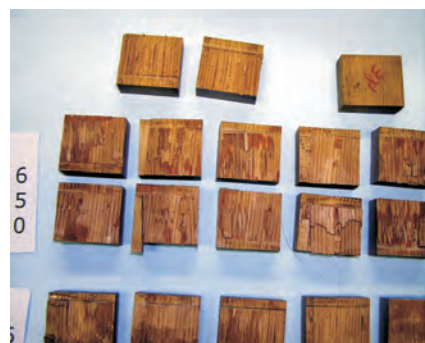
No surprises here-both the Six10 and G/flex 650 failed the wood extensively after six weeks of accelerated environmental cycling. These samples gained 16% moisture each time they sat in the hot humid environment and dried to a level 2.11% below the original moisture content coming out of the dry hut. The moisture content was 1.59% above the initial room temp/ambient humidity value at testing. The original control MC block which had been dried to -4.44% for testing sat out at room temperature in our shop here in mid-Michigan for the entire six weeks and gained back 0.77% moisture during that period.
