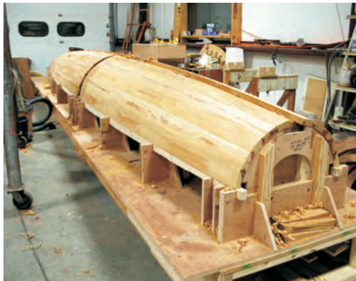
A half column is placed on a jig for fairing.
