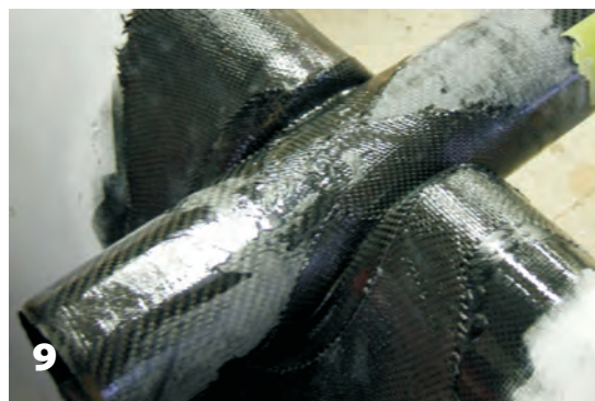
8—Carbon beams were purchased from Ben Hall and then a carbon dolphin striker was added to the front beam.
