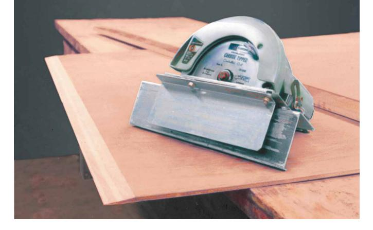
Scarfing wood together dates back ages. Scarfing is the process of cutting corresponding angles (or sometimes shapes) on two similar pieces of wood and gluing them together to create a larger piece of lumber or plywood. The most common place scarfing is used is in building a stitch-and-glue canoe or kayak.
