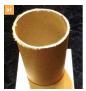
Mix a small batch of 105/207 epoxy and adhere the mailing tube to the base, allow to cure.
