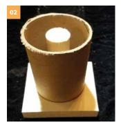
Epoxy the ¾" dowel to the base, at the center of the mailing tube.
