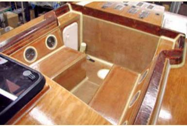
**Construction** - <sup>3</sup>/<sub>4</sub>" plywood sheathed with fiberglass and West System Epoxy
