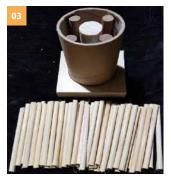
Epoxy the four darker colored dowels to the base inside the mailing tube, around the center dowel.
