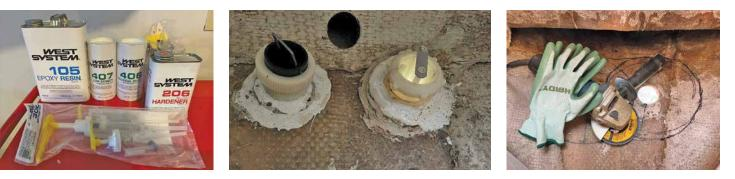
Left: Prepping our tools for the job. Middle: 2 <sup>1</sup>/<sub>8</sub>" diameter transducer thru-hulls in the bow. Right: Prepping the hull by grinding the inner glass laminate.
