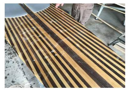
Above: The deck pads in place and the decks prepped for more epoxy before we fixed the pox.
