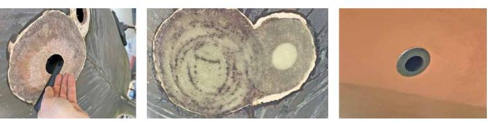
Left: We tapered the unneeded hole at a 12:1 bevel. Middle: New fiberglass patches are applied to the hull. Right: The final thru-hull after applying anti-fouling bottom paint.
