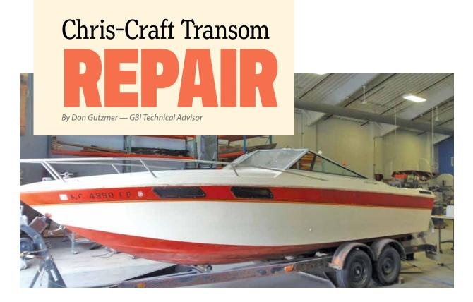
In order to demonstrate proper repair methods, our Technical Department purchased a neglected 1980 Chris Craft Scorpion 230 in need of a complete restoration. It had rotted stringers, transom, cockpit sole, and other problems common in fiberglass boats. I'll explain the process we used for replacing the transom to provide some direction on tackling similar projects.
