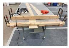
*The fence clamped to the plywood with additional secondary clamped 2"x4".*
