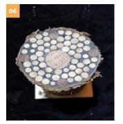
Slowly pour the epoxy mixture into tube and allow it to cure.
