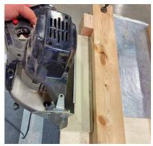
Cutting the scarf at an 8-to-1 bevel.
