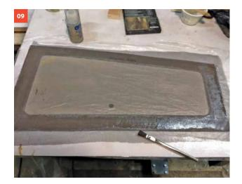
9. Flip the screen frame over, dull the backside with sandpaper, and glue in plastic window screen fabric (available at hardware or building supply stores) with G/5 Five-Minute Epoxy. Allow the epoxy to cure.
