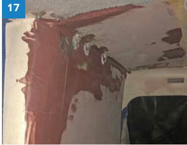
Applying the finishing touch-ups with 407 Low-Density filler to the starboard side.
