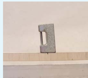
The end grain pine repair was only a little stiffer.
