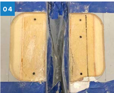
To make room for the G-10 panel, I removed the high-density foam with a router.
