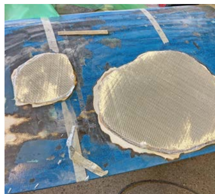
We traced the pattern on the fiberglass before cutting it out.
