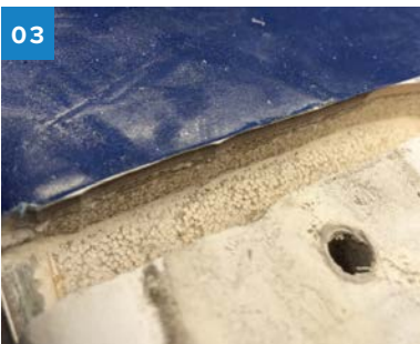
A router was the best tool for removing the high-density foam core.
