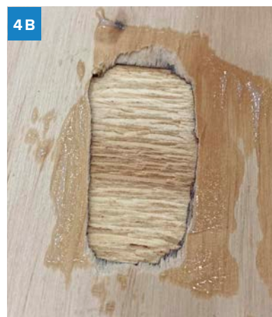
The broken (failed) surface from the plywood glued with WEST SYSTEM 105 Resin® and 207 Special Clear Hardener® thickened with 406 Colloidal Silica Filler.
