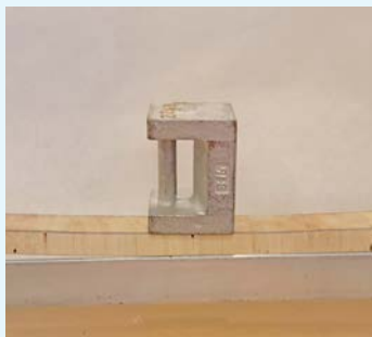
The balsa cored control sample deflected the most.
