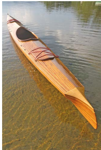
Kevin Triplett of Boston, Massachusetts designed and built this kayak using WEST SYSTEM 105 Resin, 207 Special Clear Hardener, and 403 filler.
