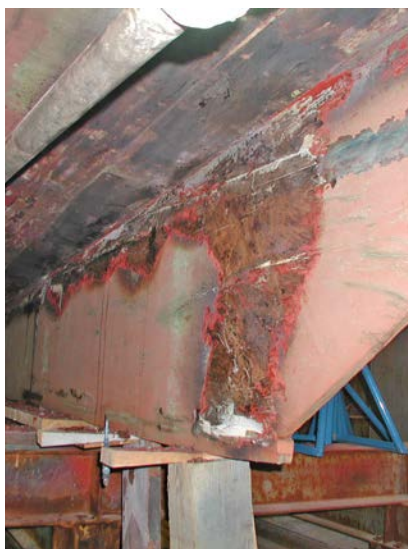
1989 keel check with epoxy repairs still good.
