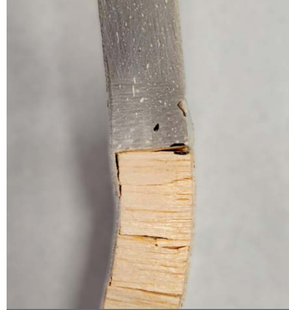
Close-up of the epoxy filled repair. Its fiberglass and balsa core fractured right at the transition from epoxy to balsa core.
